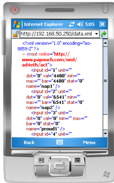
Fig. 3 Example of Opening XML file directly in the PDA via a URL address
