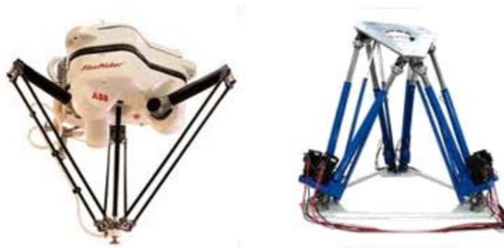
Fig. 5: Tripod and hexapod kinematic structures
