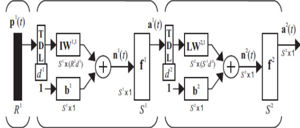
Fig.4: Distributed Time-Delay Neural Network (DTDNN)
