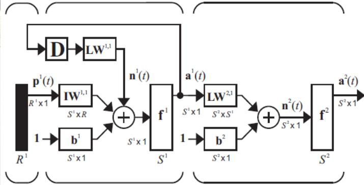
Fig.2: The Layer Neural Network (LNN)
