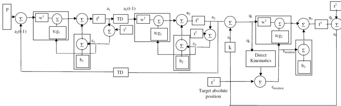
Fig.7: Detailed schema of the researched Neural Network
