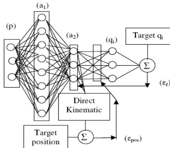
Fig.6: The proposed Neural Network. Simplified schema
