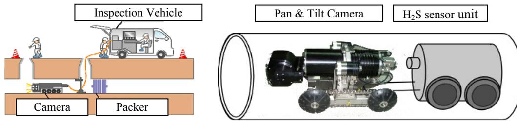
Fig. 1: Pipe inspection robot.
