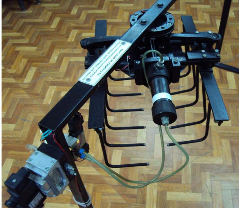
Fig. 1: Gripper for sacks manipulation
