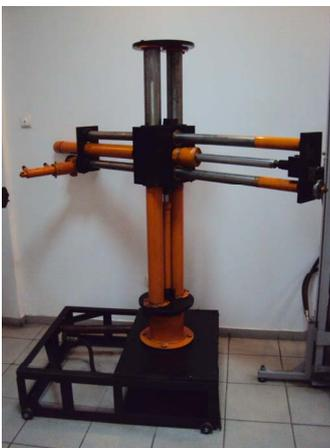
Fig. 1: The transfer manipulator
