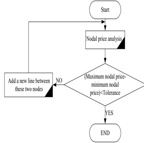
Fig. 4: The flow diagram of the new candidate lines created by the nodal price analysis
