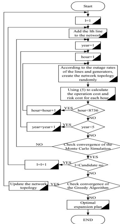
Fig. 5 The flow diagram of the method that combine the Monte Carlo Simulation and the Greedy Algorithm to find the optimal expansion plan
