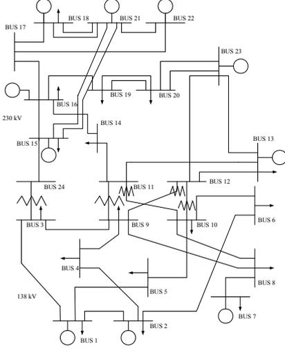
Fig. 1: The IEEE 24-bus reliability test system
