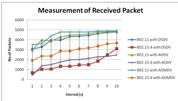
Fig. 2: Measurement of Received Packet
