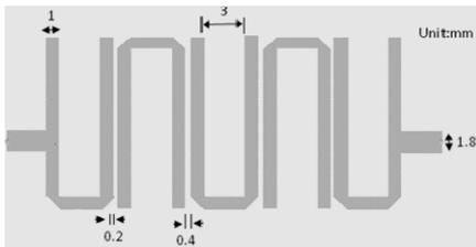
Fig. 1: Layout of conventional 5 pole microstrip bandpass filter
