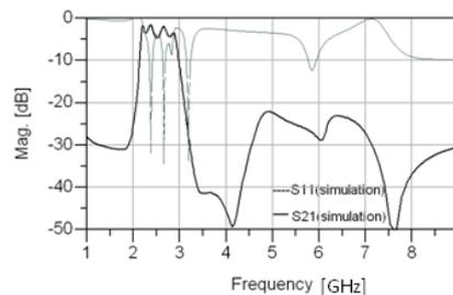
Fig. 8: Layout of B.P.F using open stub and DGS cells Fig. 9: Simulated response of B.P.F
