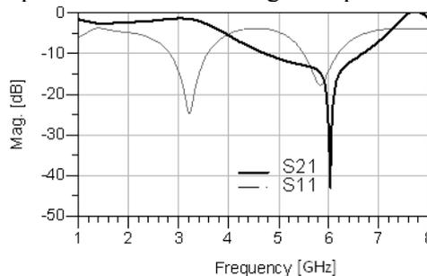
Fig. 5: Simulated response of Dumbbell DGS module
