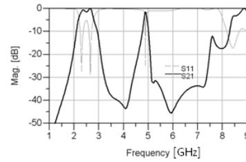
Fig. 2: Simulated response of Conventional B.P.F
