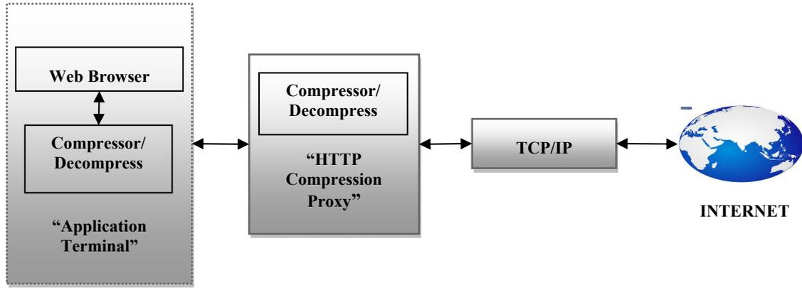
Fig. 1: Network model for web application based on HTTP Compression System
