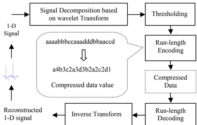
Fig. 3: Compression/ Decompression methodology based on wavelet transform and Run-length encoding
