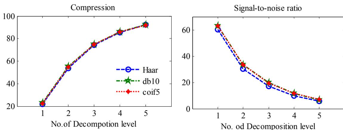
Fig. 4: Performance of different wavelet with five decomposition level for speech signal in term of *CR* and *SNR*
