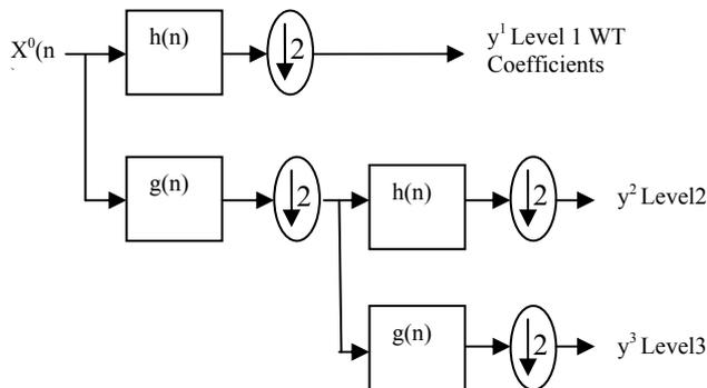
Fig.2: Filter bank representation of DWT decomposition
