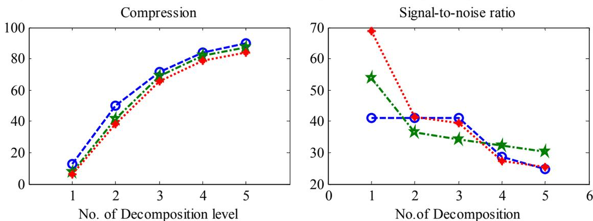
Fig. 5: Performance of different wavelet with five decomposition level for ECG signal in term of *CR* and *SNR*
