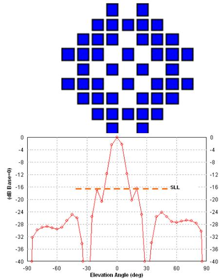
Fig. 8 Array pattern of a uniformly fed modified Sierpinski carpet based planar antenna array with shifted center elements. A peak SLL of -17 dB is observed
