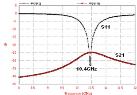
Fig.2 Return loss of two element rectangular microstrip antenna array and the corresponding mutual coupling given by S21.
