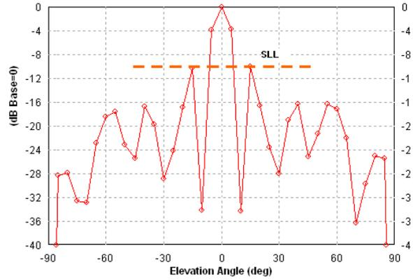
Fig. 4 Array pattern of a uniform feed 9x9 Sierpinski carpet based rectangular planar antenna array.
