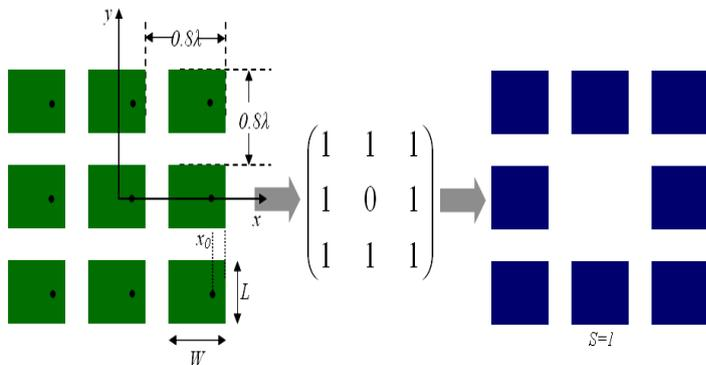
Fig.1 Illustration of the procedure for converting a 3×3 rectangular microstrip planar array in to a first stage (S=1) of Sierpinski carpet based thinned array by removing forward some
