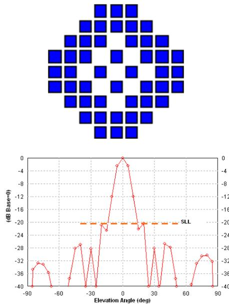
Fig. 9 Array pattern of a uniformly fed modified Sierpinski carpet based rectangular planar antenna array with shifted center elements. A peak SLL of -21dB is obtained
