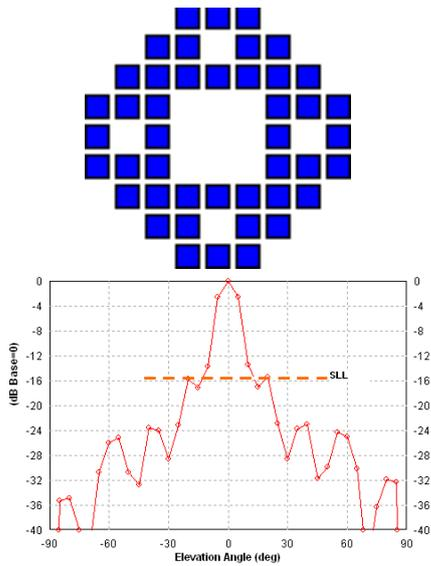
Fig. 7 Circular pattern of a uniformly fed modified Sierpinski carpet based rectangular planar antenna array with -15.5dB SLL.
