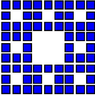
Fig. 3 Second stage of Sierpinski carpet based thinned rectangular microstrip antenna array. Lines show the central axis.
