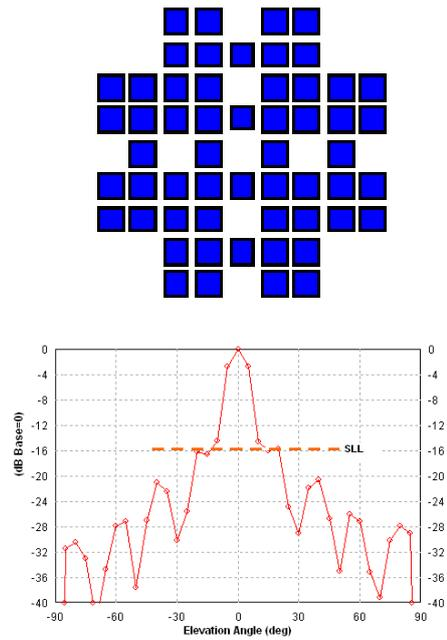
Fig. 6 Array layout after shifting elements along the central axis. A peak SLL of -16 dB is observed.
