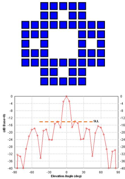
Fig. 5 Planar array layout after deleting corner elements and corresponding array pattern. A peak SLL of -14 dB is observed.
