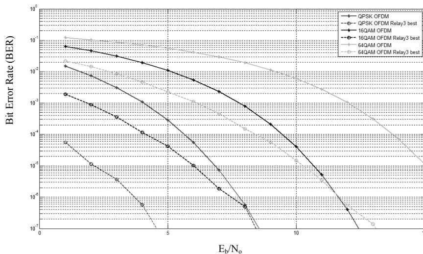
Fig. 5: Comparison of the best-relay selection schema for M-ary QAM OFDM-based system
