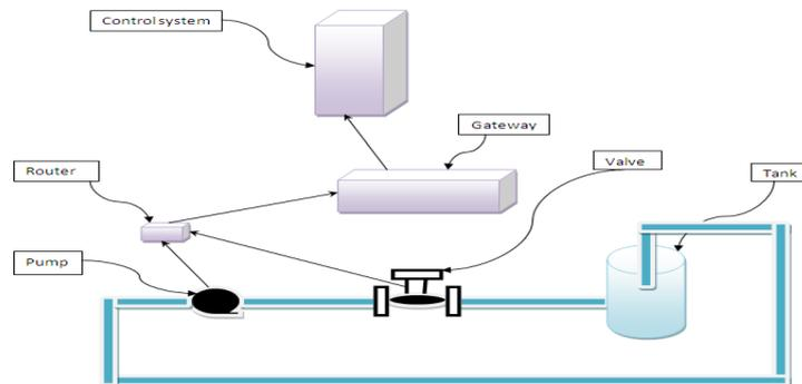
Fig 2- Schematic of a Pump-Valve system
