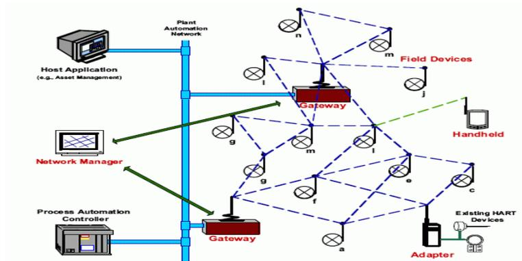
Fig. 1: Structure of a Wireless HART plant
