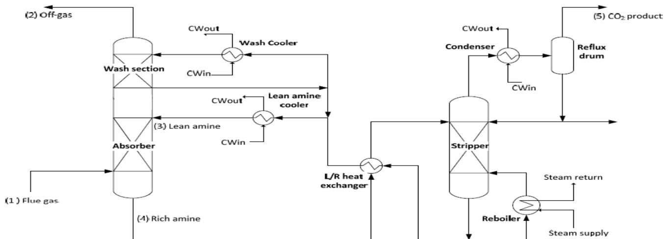
Fig. 5: Simplified process flow diagram of the CO<sub>2</sub> Capture Plant
