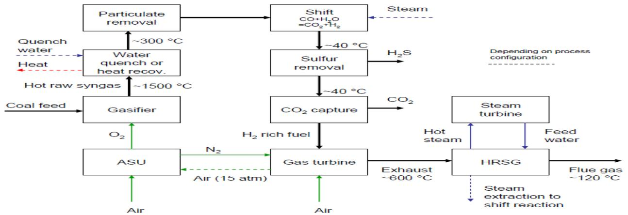
Fig. 4: IGCC Process with CO<sub>2</sub> Capture
