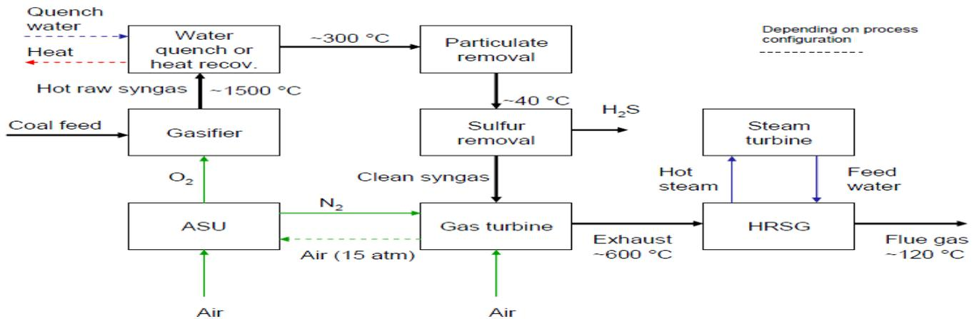
Fig. 3: IGCC Process without CO<sub>2</sub> Capture
