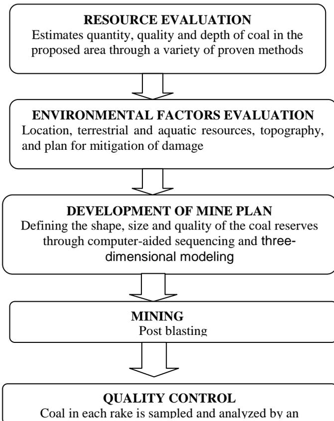
Fig.1 : Coal Mine Improvement Methodology flow diagram
