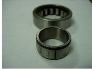
Fig.1: A rolling bearing with inner-race fault
