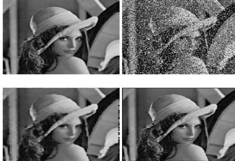
Fig. 4: Results of filtering with a 3X3 median and conditional median filter. From left to right, first row: original Image, noisy image; second row: standard median filter, Adaptive median filter.
