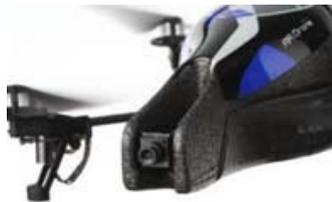
Fig. 1: Front Camera of the Drone
