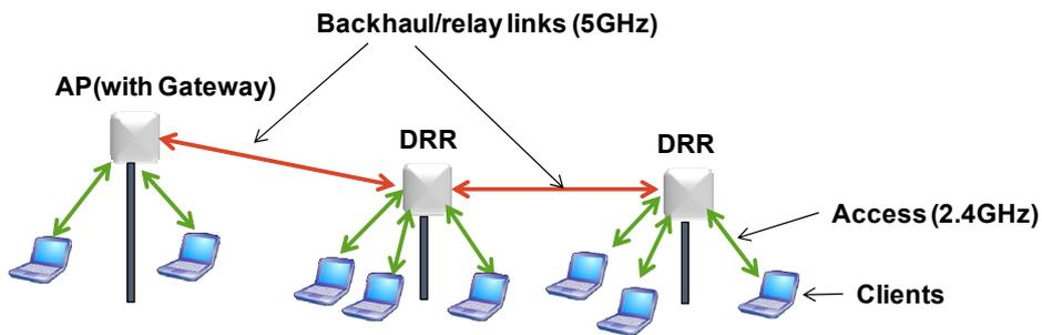
Fig. 1: Dual Radio Relay Network (DRRN) Architecture
