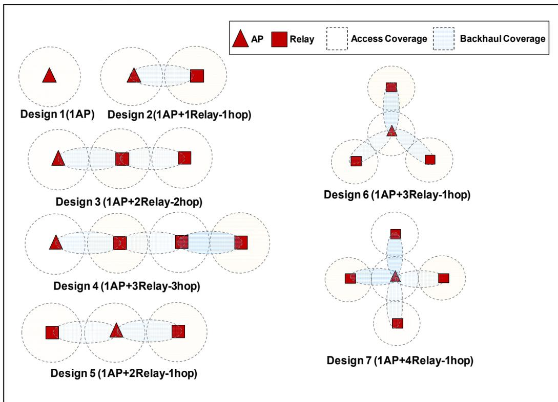
Fig. 2: Possible topologies with different number of DRR
