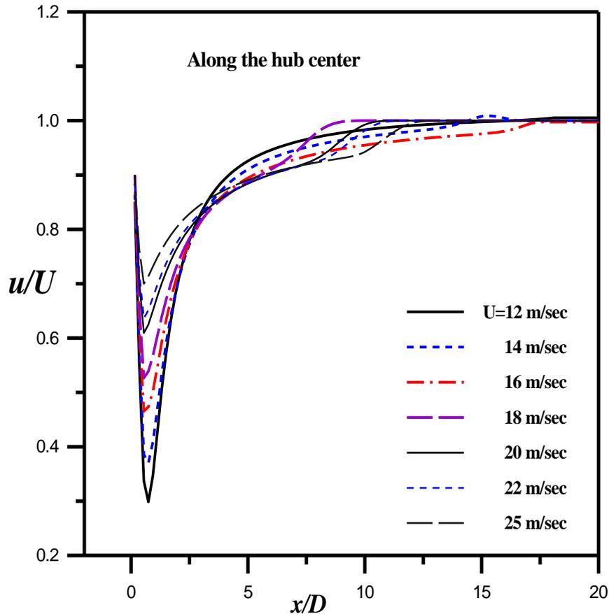
Fig. 3: Wake distribution of the 2 MW wind turbine along the axial direction at the turbine axis for different wind speeds.
