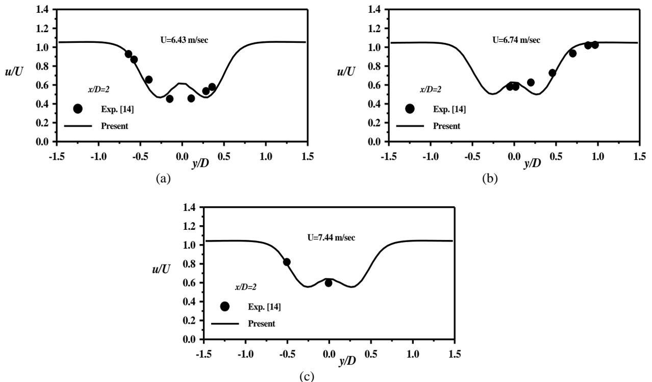
Fig. 2: Wake distribution of MOD-0A wind turbine for: (a)  $U=6.43$  and  $TI=13\%$  (b)  $U=6.74$  and  $TI=11\%$  (c)  $U=7.44$  and  $TI=13\%$ .
