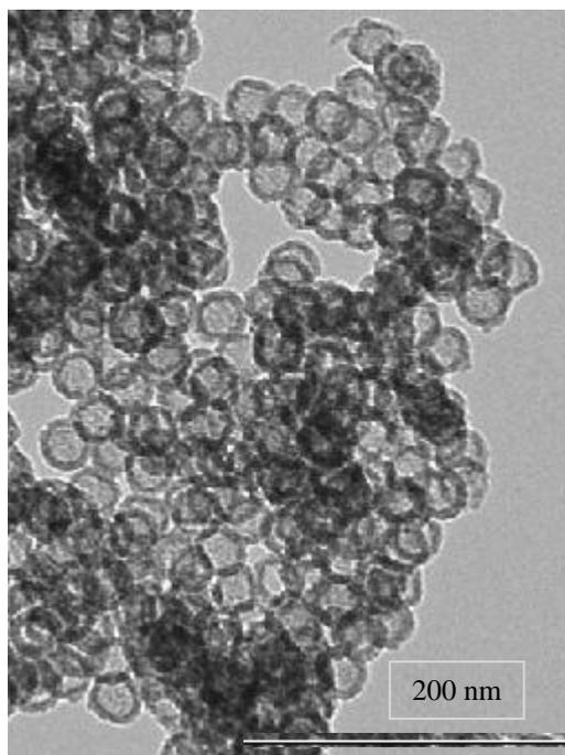
Fig. 2: TEM image of ZnO hollow nanospheres ( $Zn^{2+}/PAA = 8$ )
