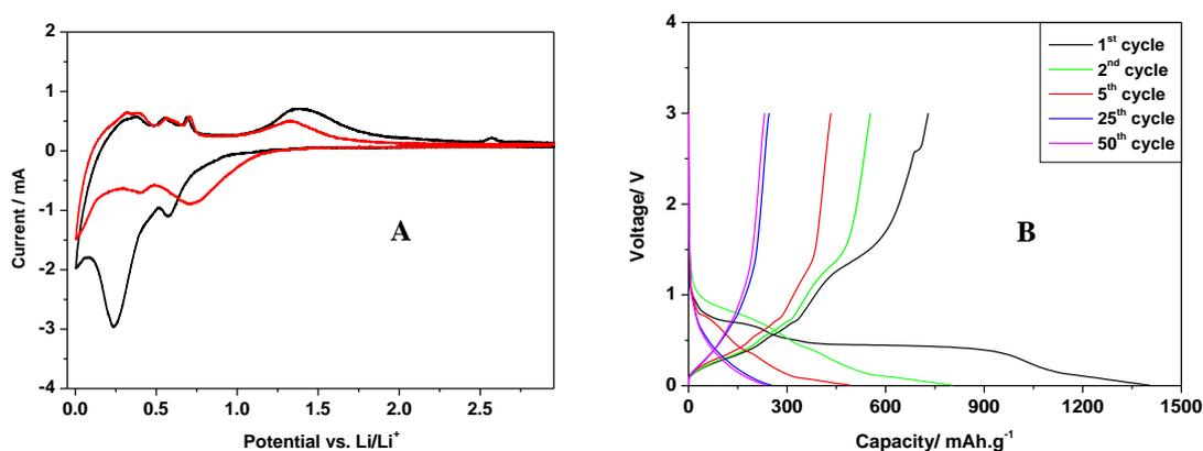
Fig. 3: (A) CV curves of ZnO hollow nanospheres in 1.0 m LiPF<sub>6</sub> (EC/DMC = 1/2 (v/v)) at a 3 mV/min sweep rate and (B) The Charge/discharge profiles ZnO hollow nanospheres at 0.25 C rate in the voltage region of 0.005-3.0 V.
