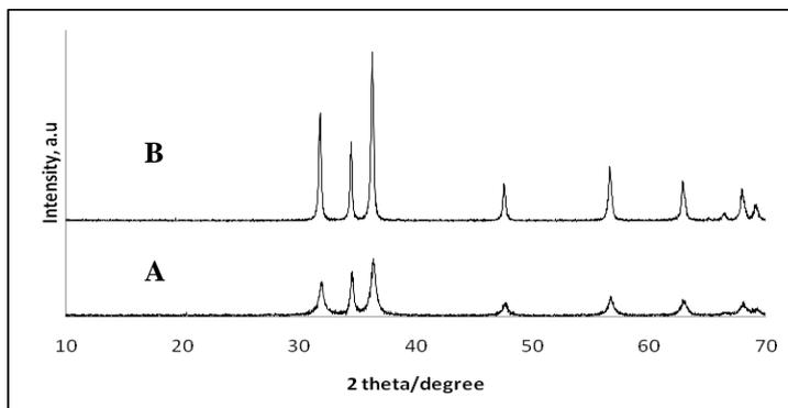
Fig. 1: Powder X-ray diffraction patterns of: (A) ZnO-composites and (B) ZnO hollow nanospheres.
