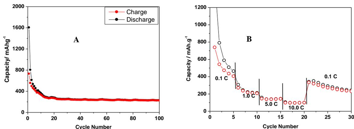
Fig. 4: (A) Charge-discharge cycling performance ZnO hollow nanospheres at 0.1 C rate in the voltage region of 0.005-3.0 V vs. Li/Li<sup>+</sup> and (B) Rate performance in the voltage region of 0.005-3.0 V.
