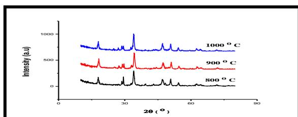
**Figure1.** XRD of the calcined egg shell catalyst calcined at different temperature.
