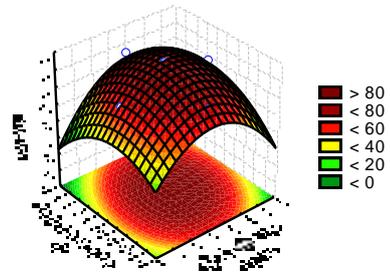
**Figure5.** Response surface curve plot showing effect of reaction temperature and methanol-to-oil molar ratio on FAME yield.
