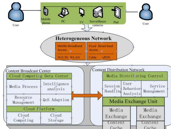
Fig.1: Multimedia field network architecture based on cloud computing
