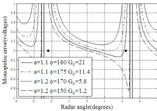
Fig. 3. Monopulse error produced by a monopulse seeker when a missile threats an aircraft.
