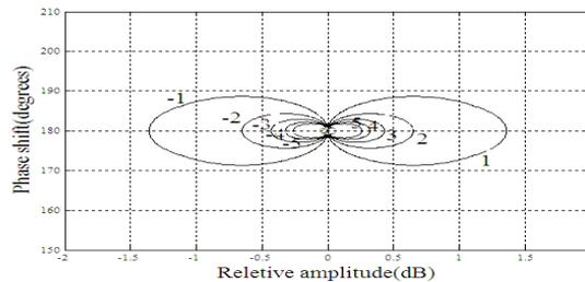
Fig. 7. Contours of monopulse error analyzed by linear fit analysis. Tolerance required to induce large angular error is strict which implies that the monopulse radar system is difficult to deceive.
