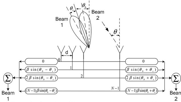
Fig. 1. Configuration of linear array antenna patterns used in amplitude-comparison monopulse system. It employs two groups of phase shifters and adders to form two monopulse beams, and an exact monopulse processor is assumed for further signal process.
