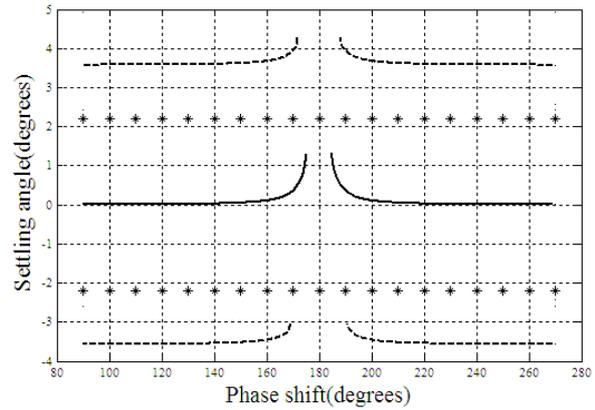
Fig. 4. Settling angle varies with the phase shift.
