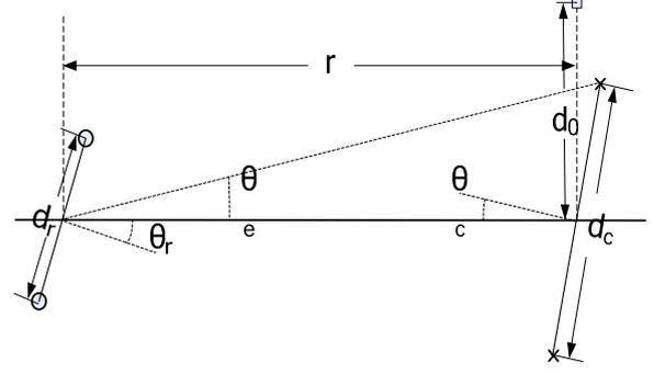
Fig. 2. The geometry of a cross-eye jamming scenario. The phase centers of the radar and jammer antenna elements are denoted by circles and crosses respectively, and the position of apparent target is shown by a square.
