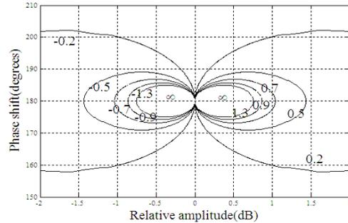
Fig. 6. Contours of monopulse error analyzed in this text. Tolerance required to induce large angular error is great which implies that the monopulse radar system can be deceived easily.
