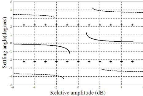
Fig. 5. Settling angle varies with the relative amplitude. Settling angle increases with relative amplitude approaches  $0dB$  which also lead to cross-eye gain increase
