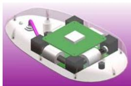
Fig.1. The integrated antenna of Loran-C H-field and GPS
