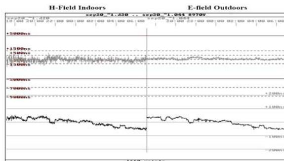
Fig.2. Comparison of ECDs (top) and TDs (bottom) from H-field antenna located indoors versus E-field antenna located on Locus' roof.
