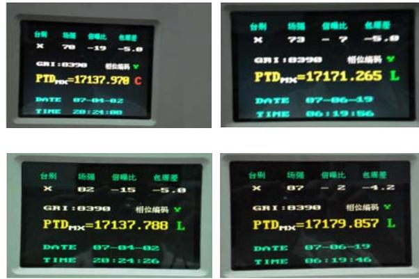
Fig.5. The real-time results of electric antenna (upside) and H-field antenna(downside)
