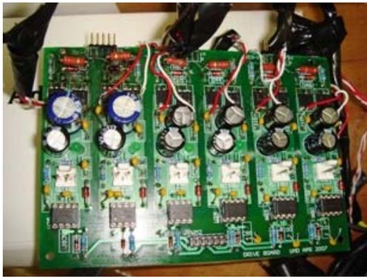
Fig.1. Real power driver board in a circuit teaching course
