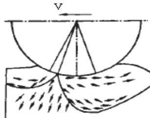
Fig.2. The flow path of sand particles
