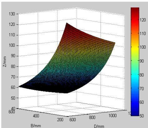
Fig.7. Subsidence changes with wheel diameter and wheel width.
