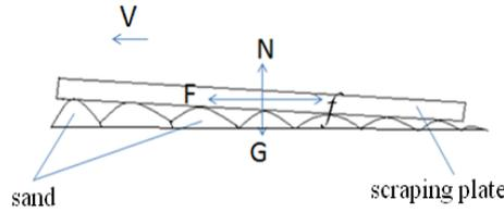
Fig.3. The force of scraping plate
