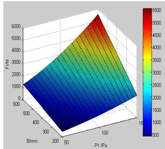
Fig.6. Compaction resistance changes with tire inflation pressure and wheel width.
