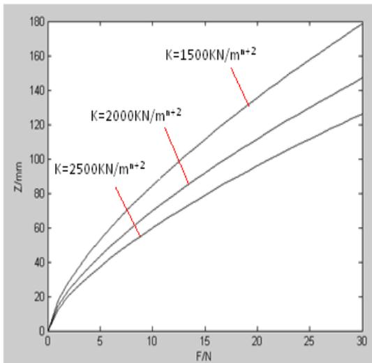
Fig.5. Modulus of deformation impact on load - Subsidence
