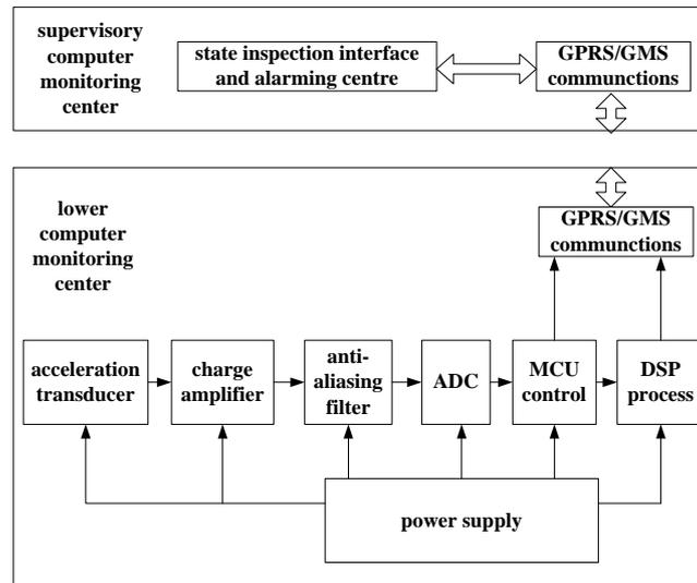
Fig.2. System construction diagram
