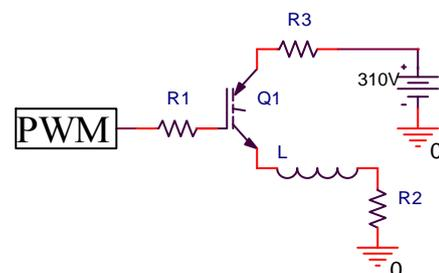
Fig. 2. Simulation model in Pspice
