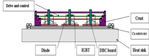
Fig.4. Schematic of typical module structure
