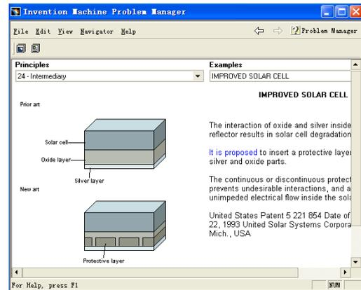
Fig. 9: An application case of Principle 24
