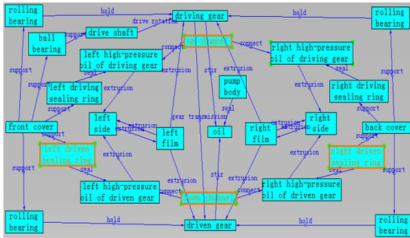
Fig. 10: The functional model of the improved gear pump
