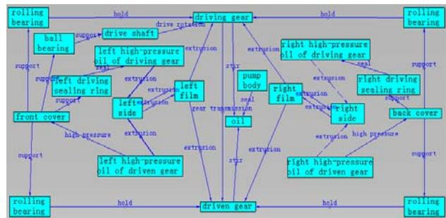
Fig. 3: The functional model of the original gear pump
