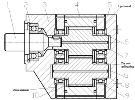
Fig. 11: The schematic diagram of the improved gear pump
