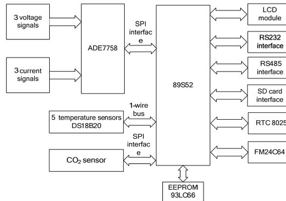
Fig.1. Hardware block diagram of the monitoring system.
