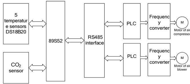
Fig.2. Hardware block diagram of the control system
