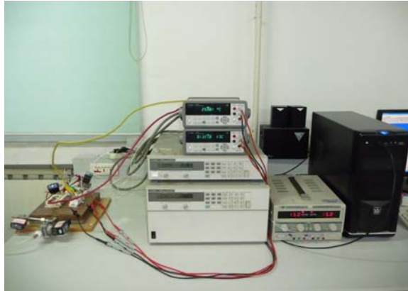
Fig.6 Platform for IGBT thermal resistance test
