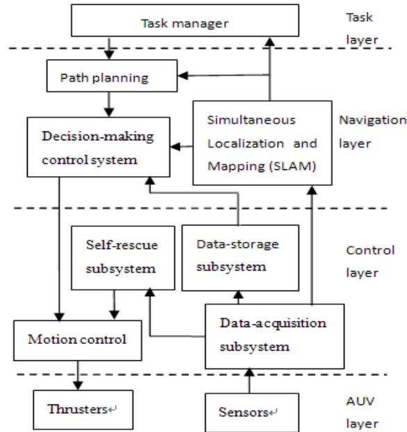
Fig.1. the block diagram of the whole AUV's system
