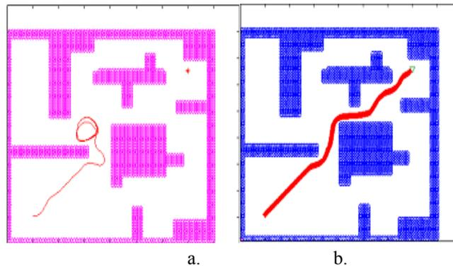
Fig.6. the simulation result of decision-making control system: a) based on the traditional APF. b) based on the improved APF
