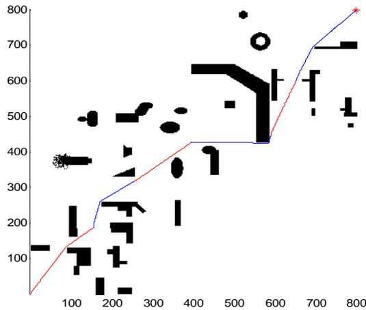
Fig.4. the simulation result of FM based path planning: the optimal path on complex obstacle map (800×800 pixels)
