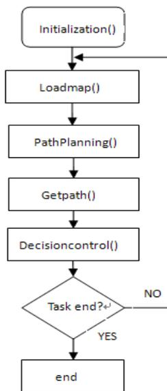
Fig.7. software flow chart of path planning and decision-making control system.
