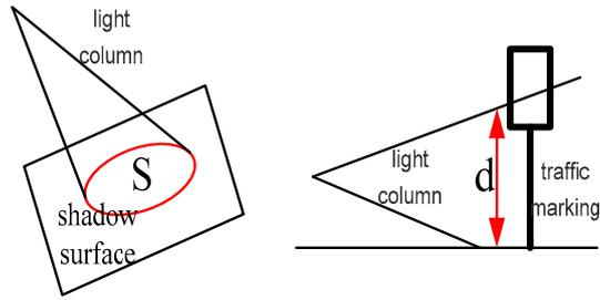
Figure 6 Illumination range and illumination height
