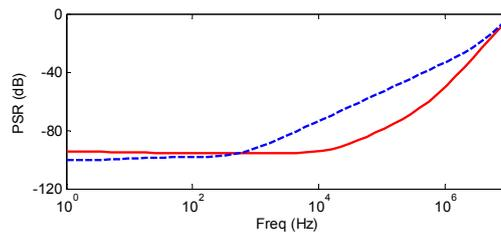
Figure 7. Comparison of PSR between LDOs with and without FFC with 0.5mA load current.
