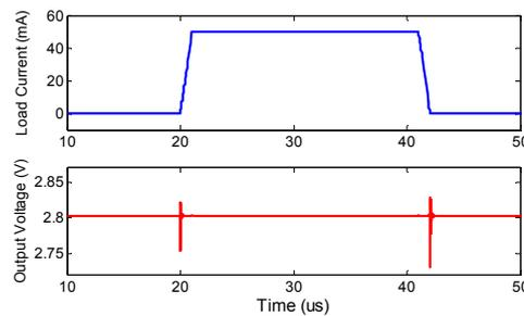
Figure 8. Load transient response of the proposed LDO.
