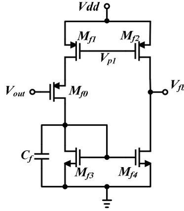
Figure 3. FFC circuit structure
