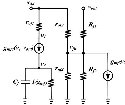
Figure 4. Small signal mode for PSR of FFC circuit
