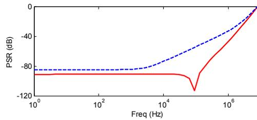
Figure 6. Comparison of PSR between LDOs with and without FFC with 50mA load current.
