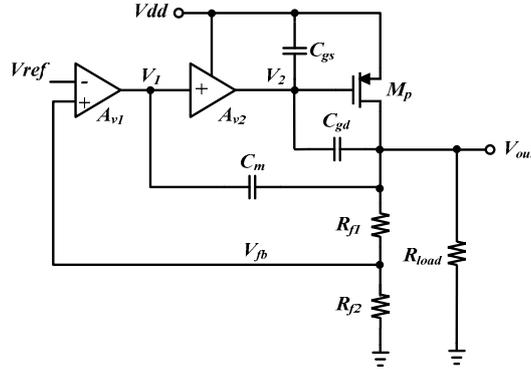
Figure 2. Basic LDO regulator with traditional NMC structure circuit
