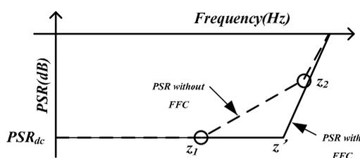
Figure 1. The PSR characteristics diagram with FFC and without FFC
