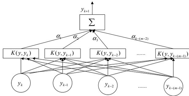
Fig.1 Topological structure of time series model on LSSVM
