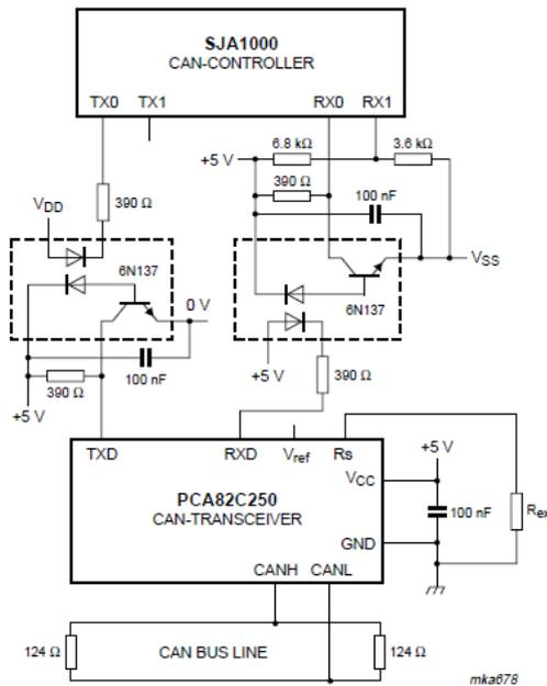
Figure 5. CAN drive circuit design
