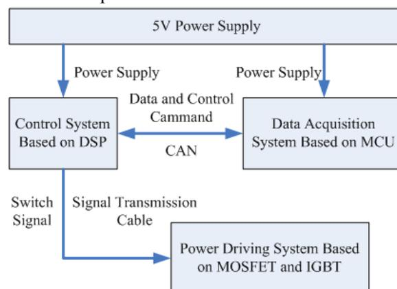
Figure 1. Structure of PMSM driving system
