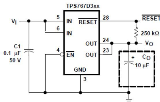
Figure 2. Power supply circuit with TPS767D318
