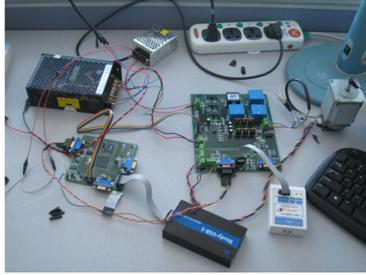
Figure 7. 24V/12W PMSM driving system
