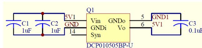
Figure 6. Isolation power supply design
