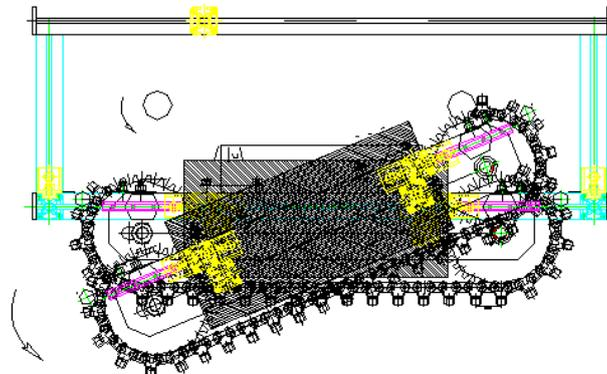
Figure. 6 Rotational walking structure of WCRSRR
