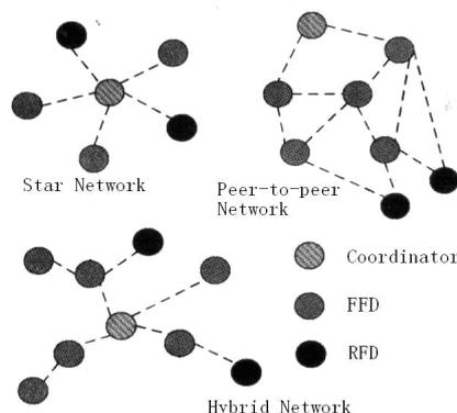
Figure.1 Structure diagram of Zigbee network connection
