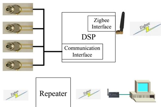
Figure.2 The structure of temperature measurement system
