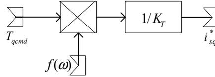
Figure 5. Block diagram of torque controller
