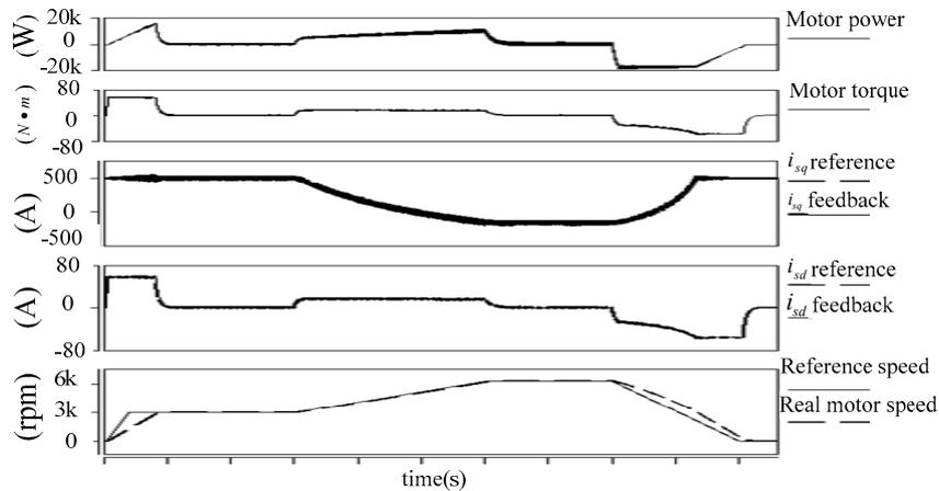
Figure 8. Motor dynamic response on the level ground
