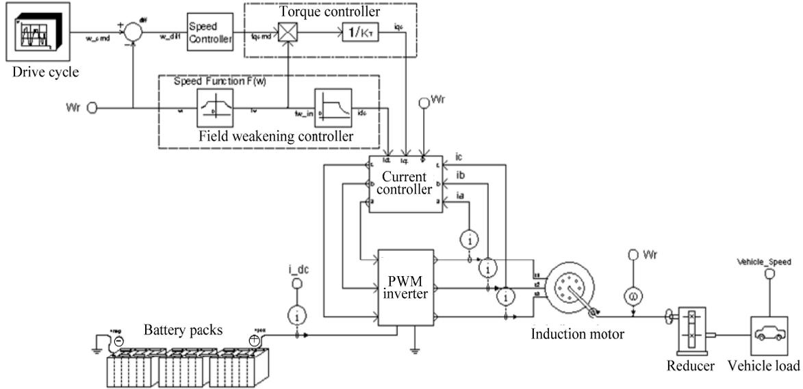
Figure 7. Block diagram of EVs propulsion system simulation model
