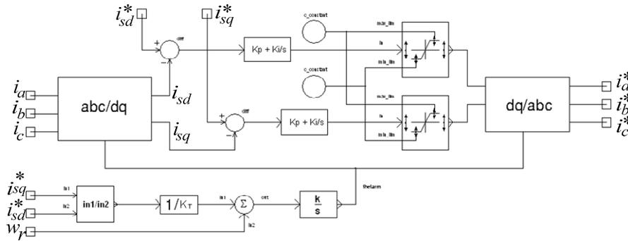
Figure 6. Block diagram of current controller
