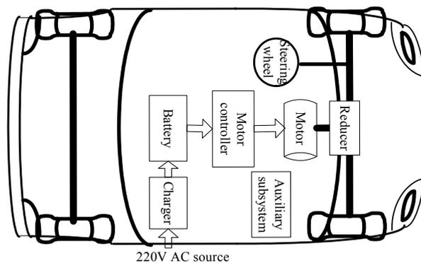
Figure 2. Typical EV system structure
