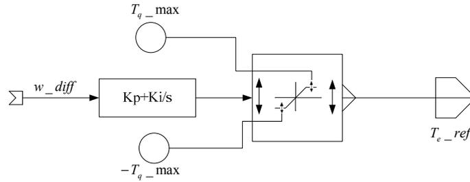
Figure 4. Block diagram of speed controller
