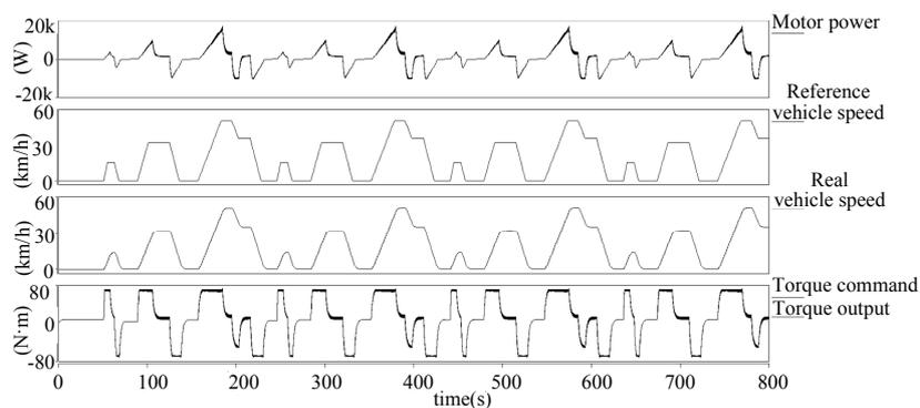
Figure 10. Simulations results of drive cycle ECE-15
