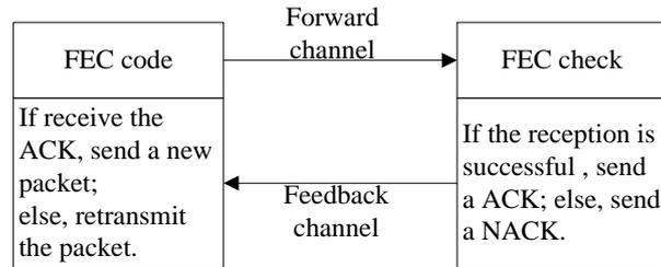
Fig. 1. Block diagram of HARQ principle.
