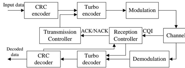
Fig. 5. System model of improved HARQ scheme.
