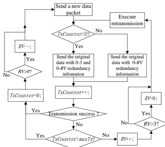
Fig. 3. Flow chart of the improved transmission controller.
