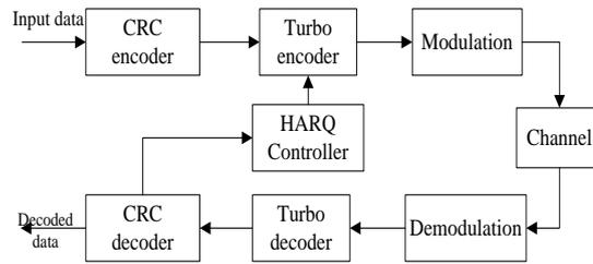
Fig. 2. HARQ system diagram.
