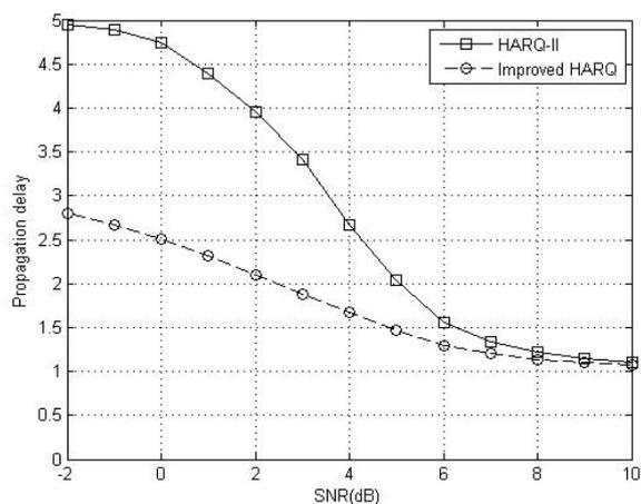
Fig. 7. Propagation delay comparison of the improved HARQ with type II HARQ, under AWGN channel.
