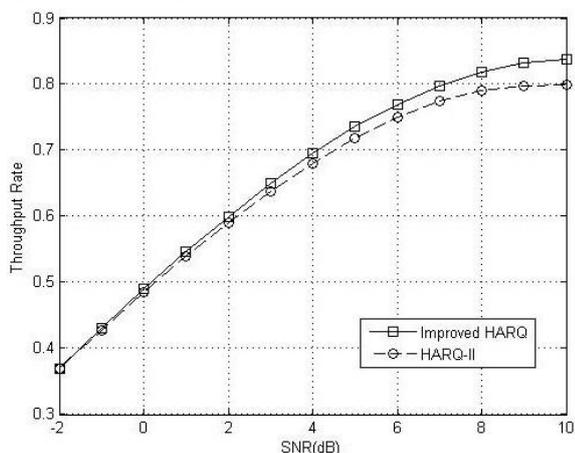
Fig. 6. Throughput rate comparison of the improved HARQ with type II HARQ, under AWGN channel.
