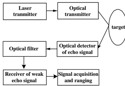
Figure 1. Block diagram of the laser ranging system
