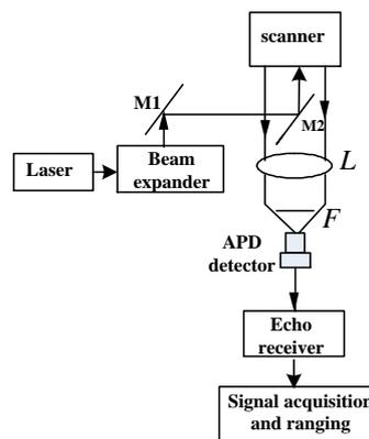
Figure 2. Optical schematic of laser ranging system
