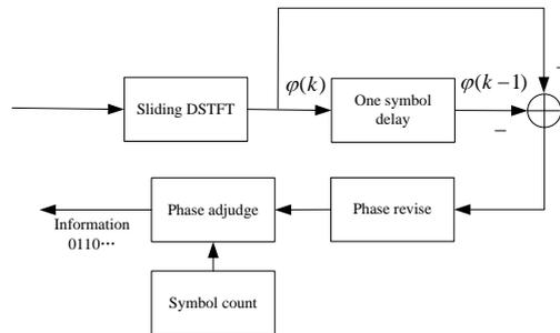
Figure 1. Demodulation block diagram
