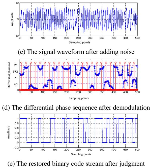
Figure 2. The waveform of modulation and demodulation system
