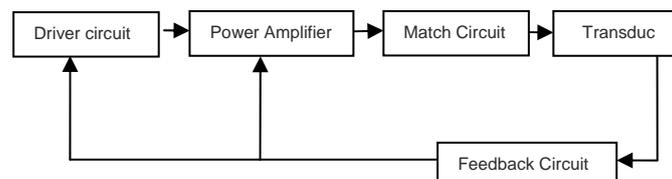
Fig. 1: Principle of Ultrasonic Generator
