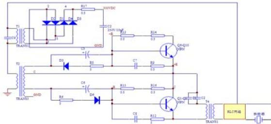
Fig.5.1: Power Feedback Circuit.
