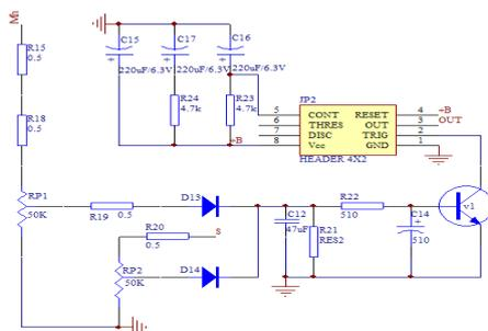
Fig.6.1: Time Base Electric Circuit.
