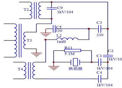
Fig.5.2: Power Feedback Circuit.
