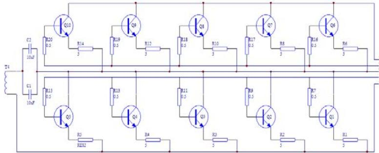
Fig.4: The Structure of Lord Amplifier Circuit
