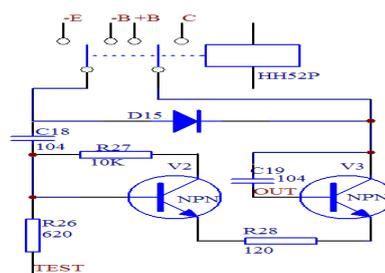
Fig.6.2: Control Signal Circuit.
