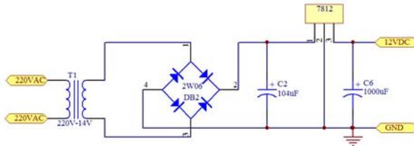
Fig.3: 12V DC Circuits
