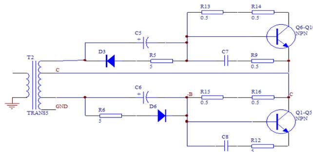
Fig.6.3: Drive Circuit
