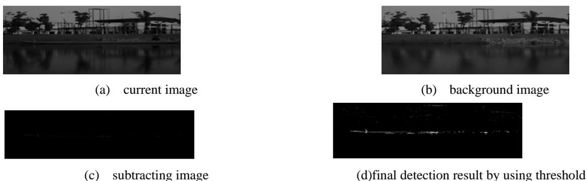
Fig. 1: Example of using Background subtraction.
