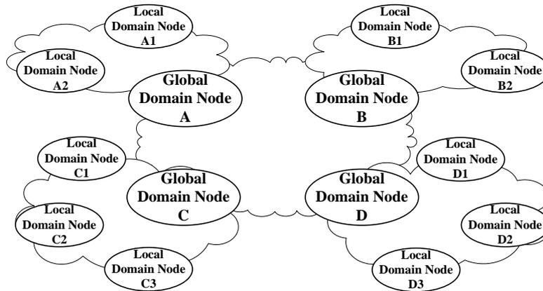
Fig. 3. Global Distributed Deployment Framework
