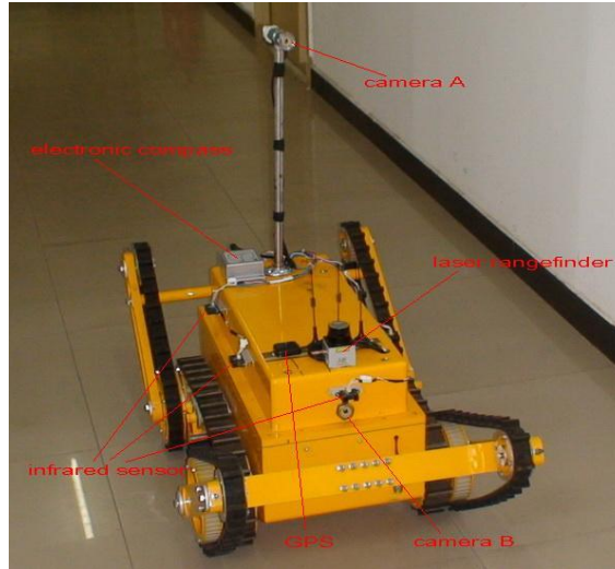
Figure 2. The physical structure of the tracked AMR
