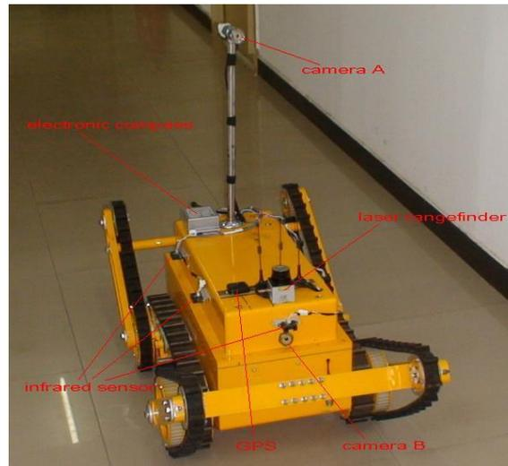
Figure 2. The physical structure of the tracked AMR
