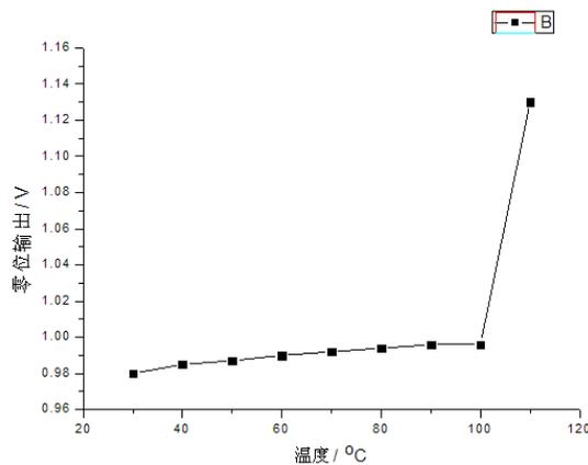
Figure 3.17 high-temperature stepping test results
