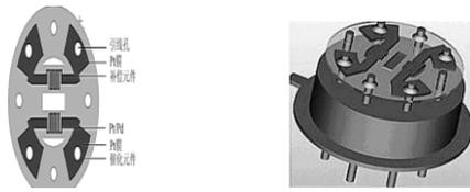
(a) Sensor chip (b) Sensors structure
