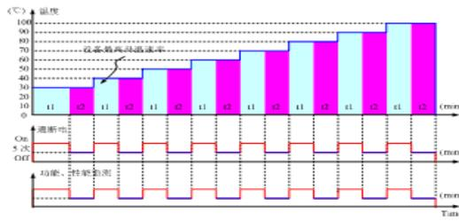
Figure 3.2 high-temperature stepping test section
