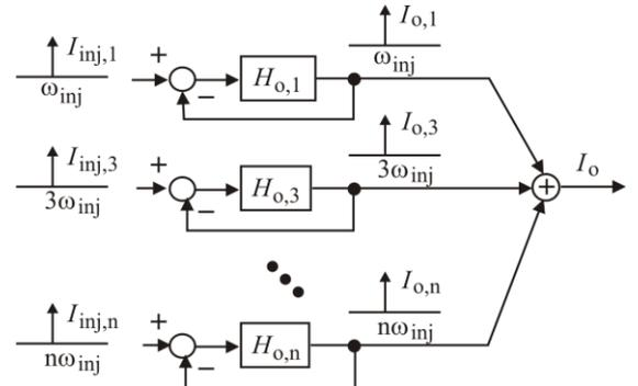
Figure 2: Representation of injection-locked non-harmonic oscillators with injection-locked harmonic oscillators.
