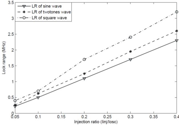
Figure 5: Simulated dependence of lock range (LR) of relaxation oscillator on injection strength and the number of frequency components of the injection signal.
