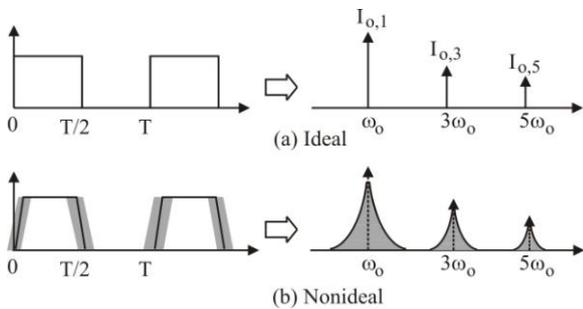
Figure 1: Time-domain waveform and spectrum of non-harmonic oscillators
