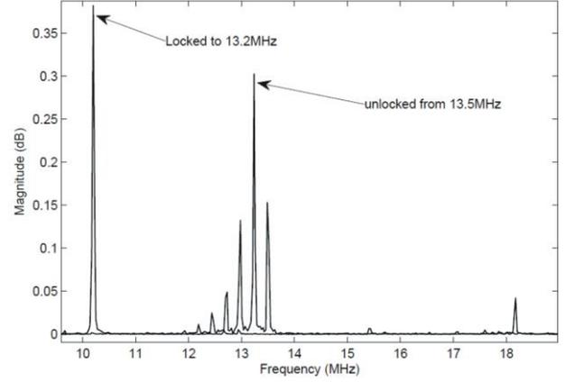
Figure 4: Simulated spectrum of the oscillator in lock state. The spectrum of the oscillator in the lock state is left-shifted by 3 MHz for a better view.  $I_{inj} = 12.65\text{ nA}$  and  $I_o = 126.5\text{ nA}$ , i.e. injection ratio=0.1.
