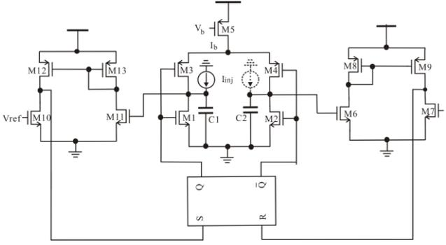
Figure 3: Schematic of relaxation oscillator with injection-locking. Circuit parameters:  $W_{1,2,6,7,10,11} = 0.5\mu\text{m}$ ,  $W_{3,4} = 1.2\mu\text{m}$ ,  $W_{8,9,12,13} = 1.25\mu\text{m}$ ,  $W_5 = 2\mu\text{m}$ ,  $V_{ref} = 310\text{ mV}$ ,  $I_b = 253\text{ nA}$ ,  $V_b = 620\text{ mV}$ .
