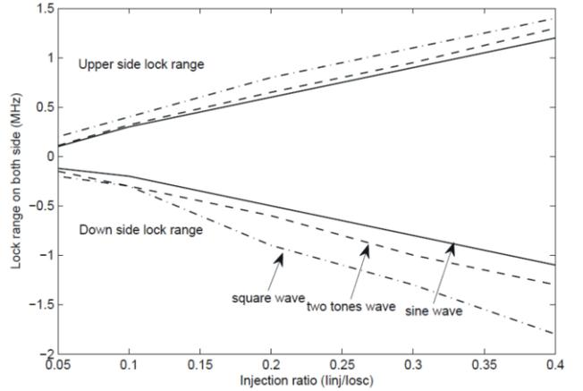
Figure 6: Asymmetry of lock range of relaxation oscillator.
