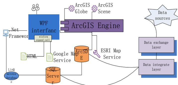
Fig. 1 High level system architecture
