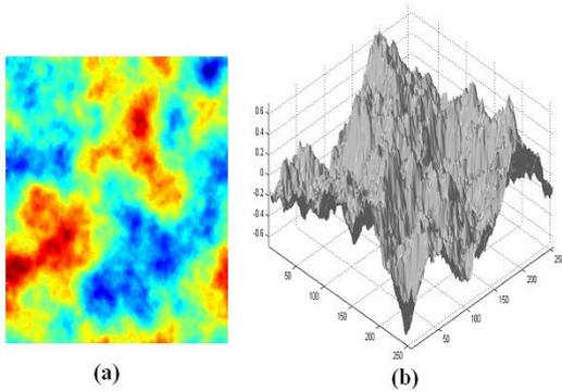
Fig.1: Phase screen function by sampling Kolmogorov spectrum and its surface plot ( $r_0=1$ ).
