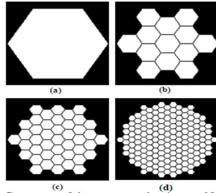
Fig.2: Geometry of the segmented mirror **a-** $N_h=1$ . **b-**  $N_h=13$ . **c-**  $N_h=43$ . **d-**  $N_h=169$ .
