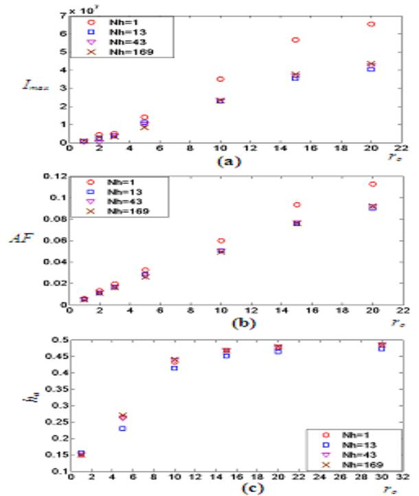
Fig. 7: **a-**The height of psf versus  $r_o$ . **b-**Average MTF versus  $r_o$ . **c-**  $h_a$  versus  $r_o$ .
